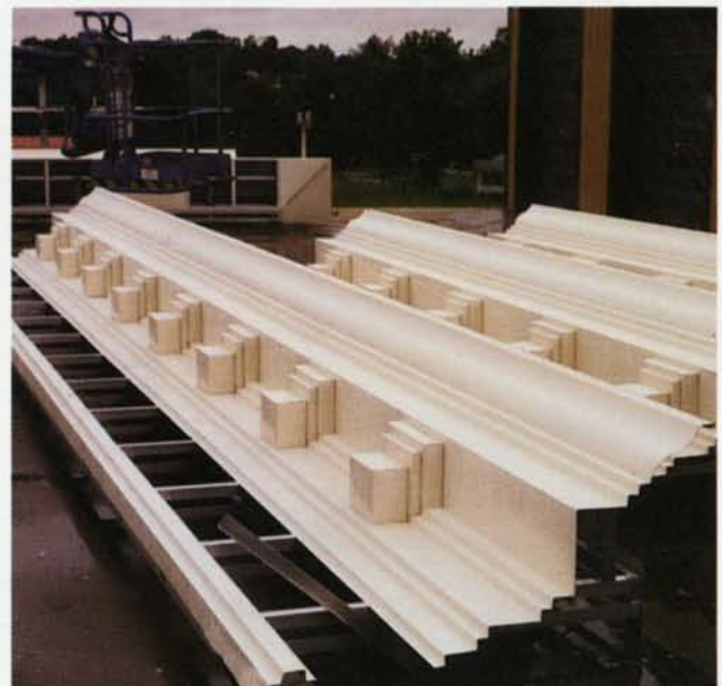
Aluminum Cornice with Aluminum Framework Awaiting Delivery
